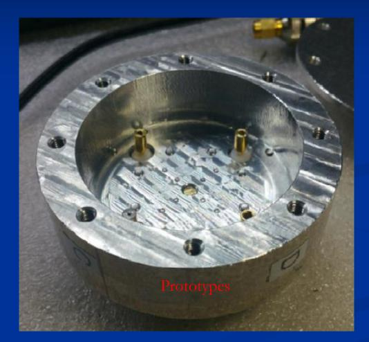
Antenna: L = 6,5mm Diameter = 3mm Distance to Body = 2mm
