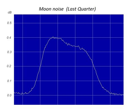
Receiver: There are some reserve there. I use not very new chips by UMS in LNA and now it is possible to improve it. I hope it can be improved from 5dB to 3dB noise figer. Also it is possible to try cooling. But there is also a limit. Antenna noise temperature is fully determined by moon noise. If to add atmosphere loss noise we get more then 200K for antenna and this is a limit.
