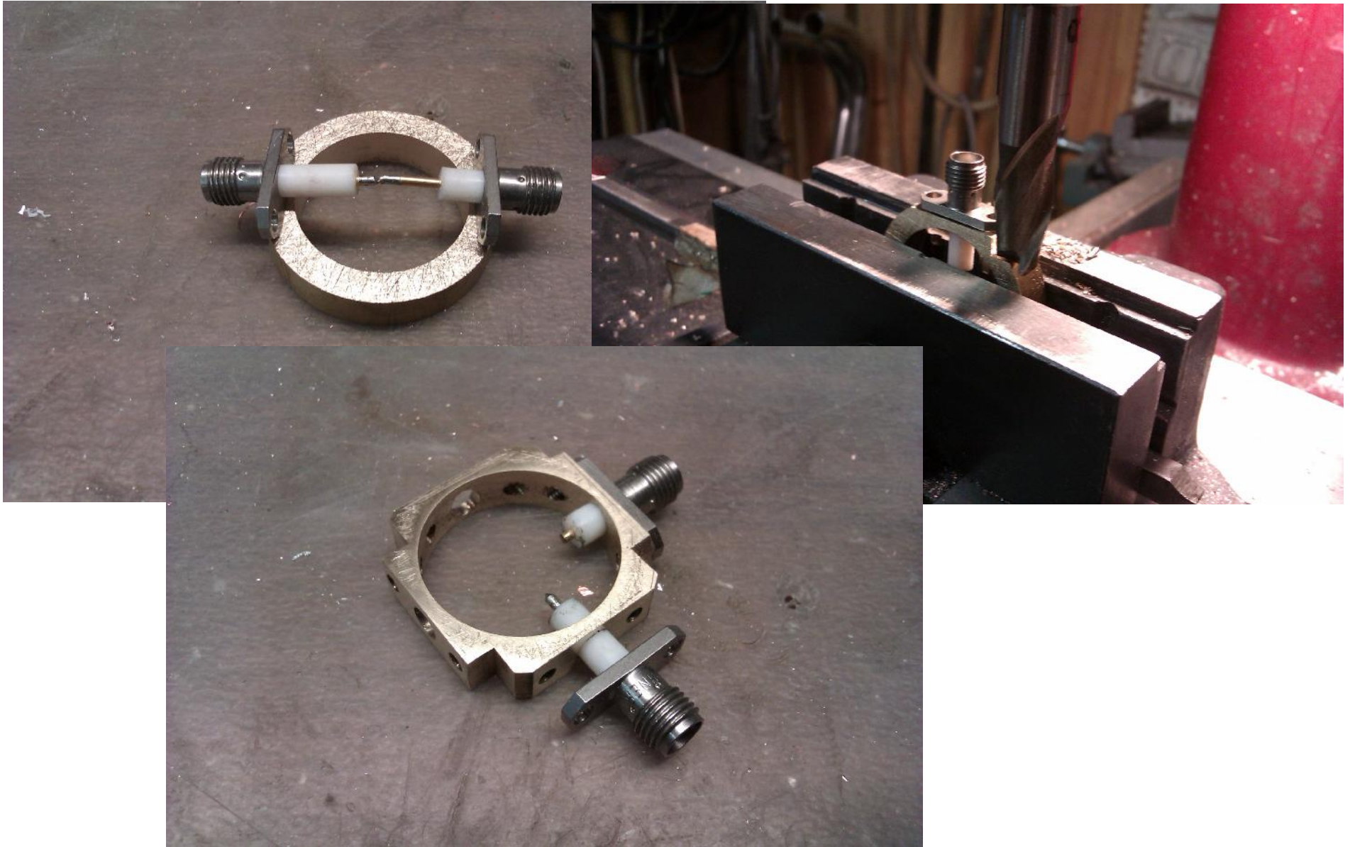
SMA connector fittings made in another way, in this case for two hole connectors
