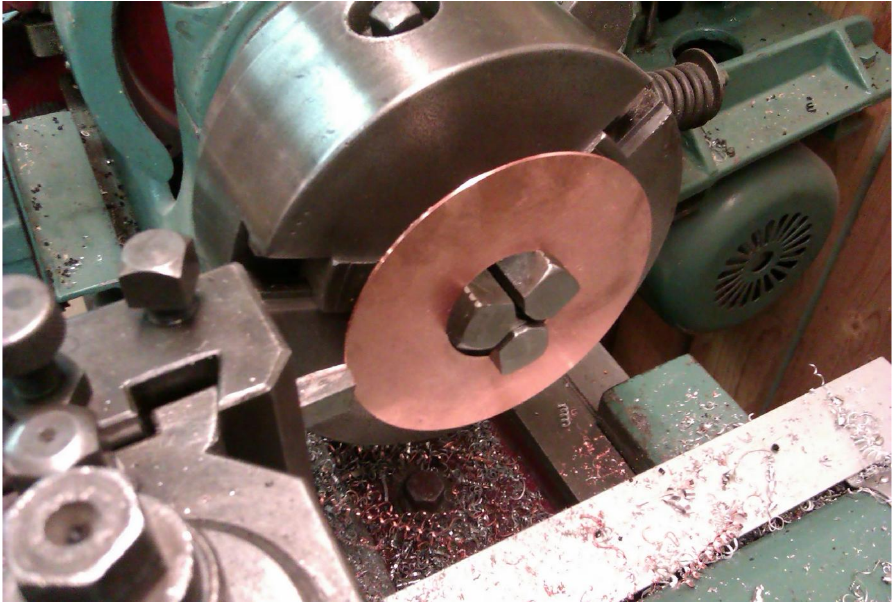
Turning the outer diameter
