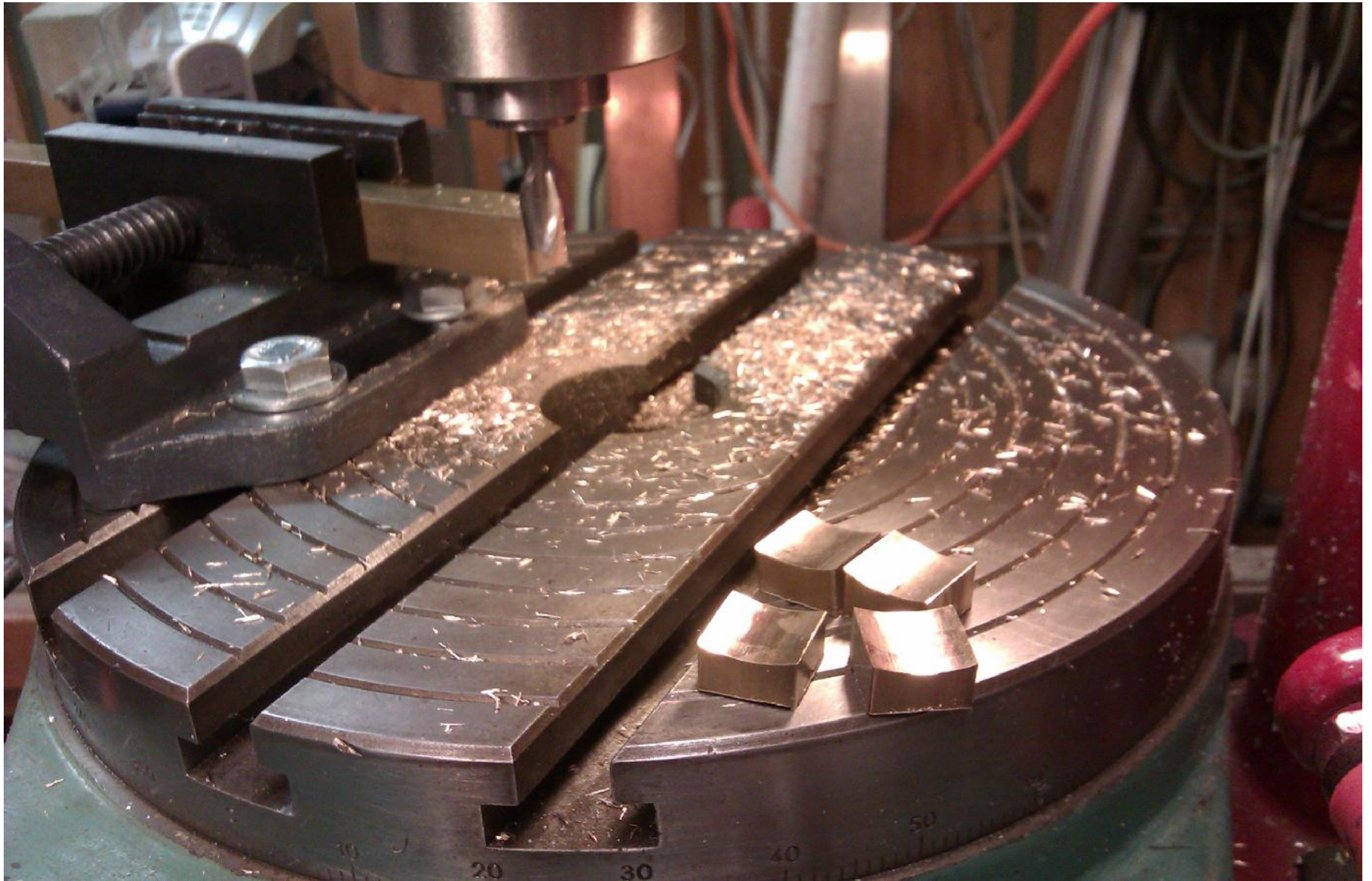
Milling radius at the SMA connector fittings, 15 x 15 mm brass
