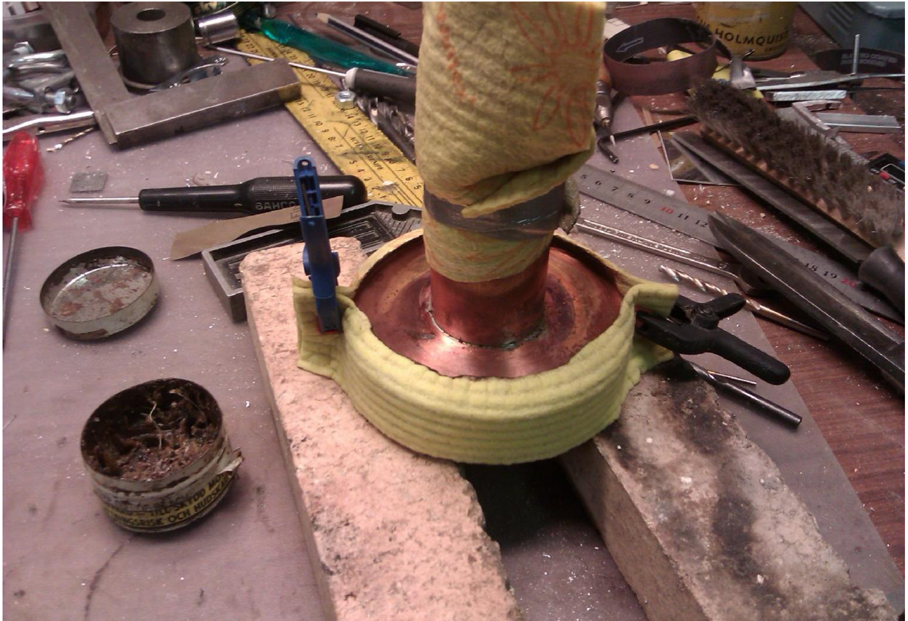
Soldering the Choke assembly to the WG.
